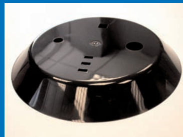
MOULDED WITH RTC™ – same ABS material, same material temperatures but much reduced injection pressure to give a high gloss finish on the 'A' surface and no visible weld lines.
