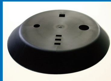
CONVENTIONALLY MOULDED – matt ABS at 2mm wall thickness, with normal material temperatures and mould temperatures of 60°C.
